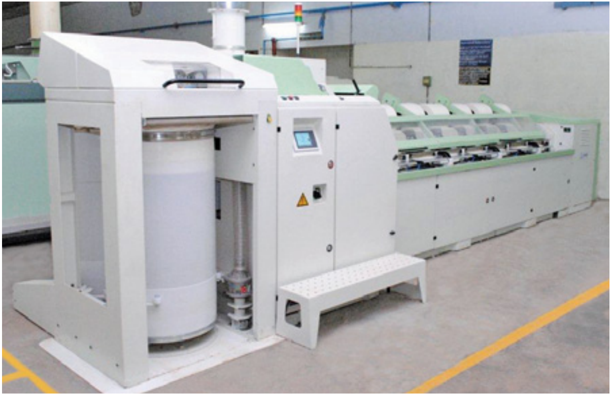
A view of the new LK64z Comber Machine installed at our Mill.
