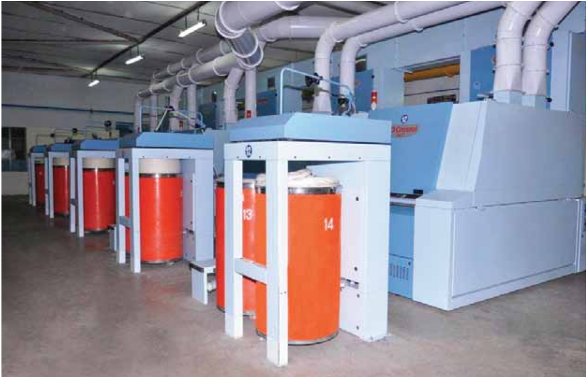
A view of the new Crosrol MK7 Carding Machine installed at our Mill.
