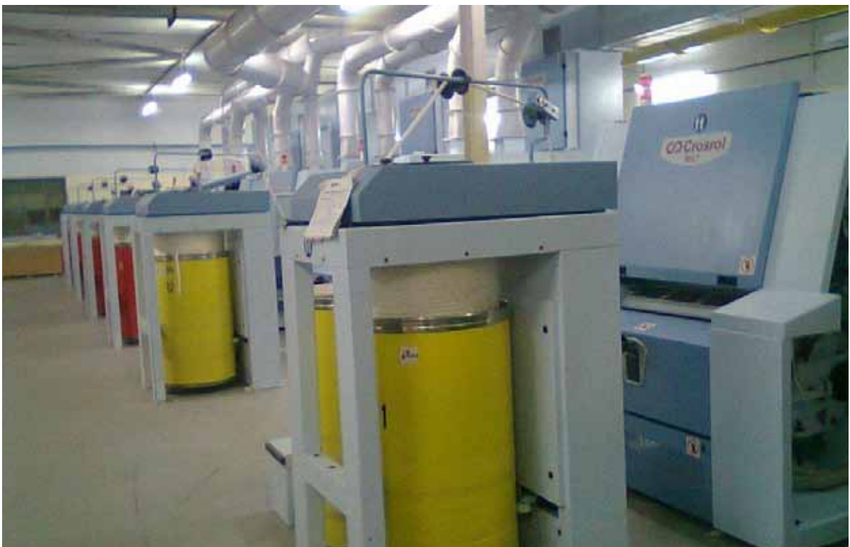
A view of the new Crosrol MK7 Carding Machine installed at our Mill.
